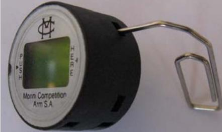
Insert the new battery (type CR2032). It can be inserted only in one position (see picture).
