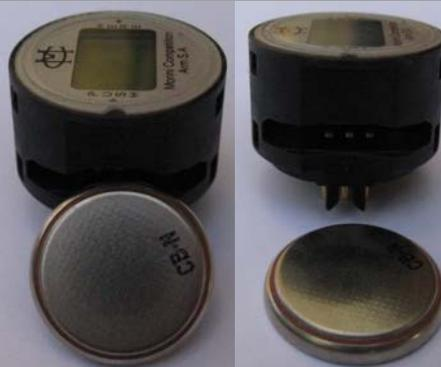
Please check that the contacts are clean before inserting the manometer. The contacts are gold plated and cannot be touched (oxidation).
